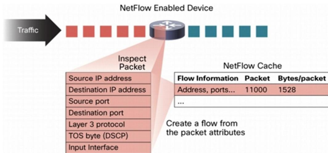
Figure 2: IP traffic flow. Copied from Cisco Network Management System (2007) [6]
