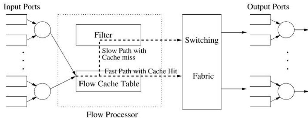
Figure 3: Flow processor. Copied from Ye Tung (2001) [12].
