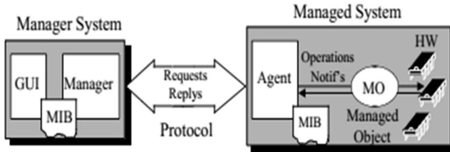
Figure 1: NMS architecture. Copied from Network Management in IP Networks [5, 19].
