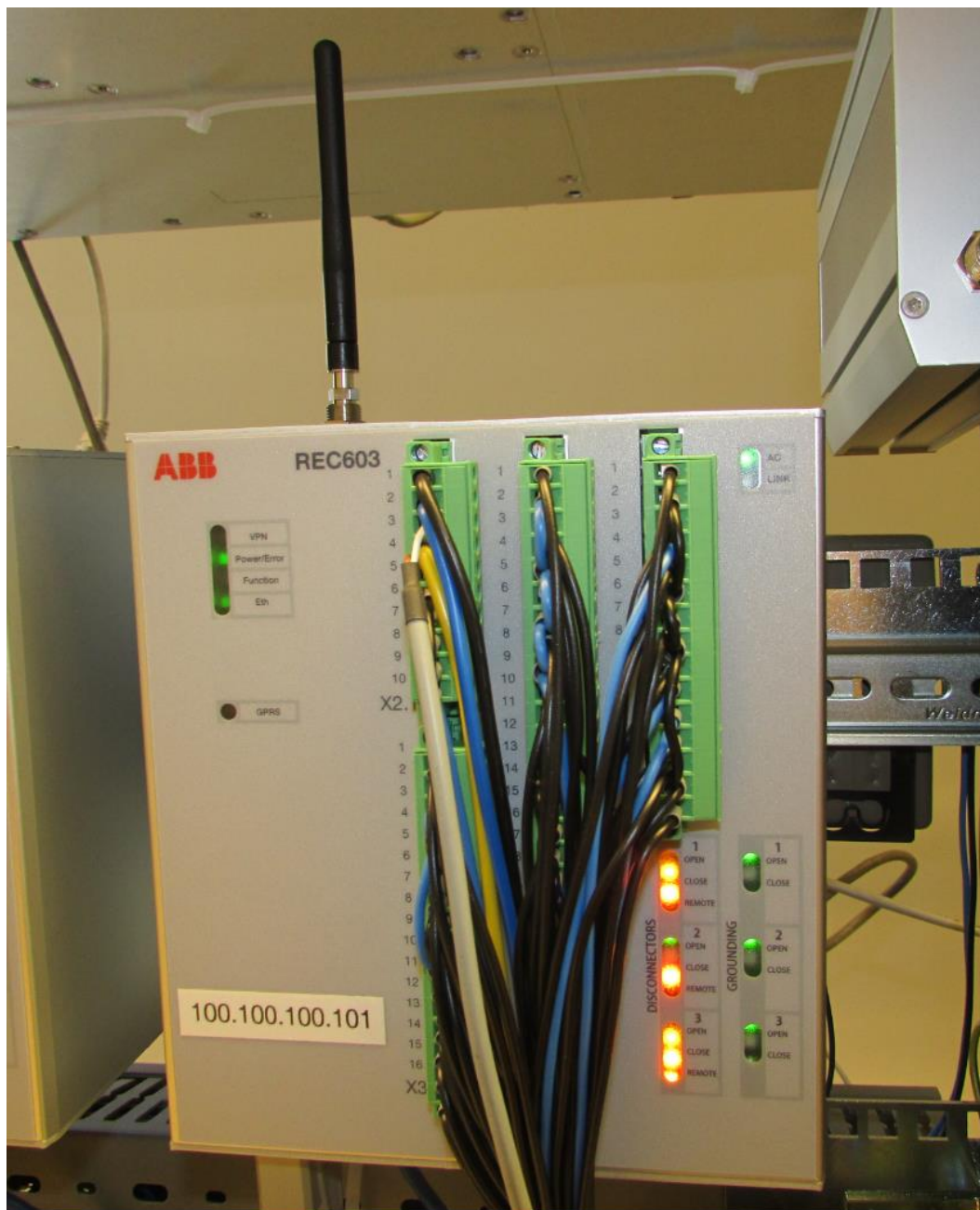
Figure 16. REC603 wireless control unit in action.
