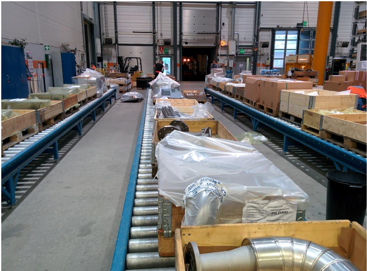
Figure 9. Roller conveyors and unloading docks
