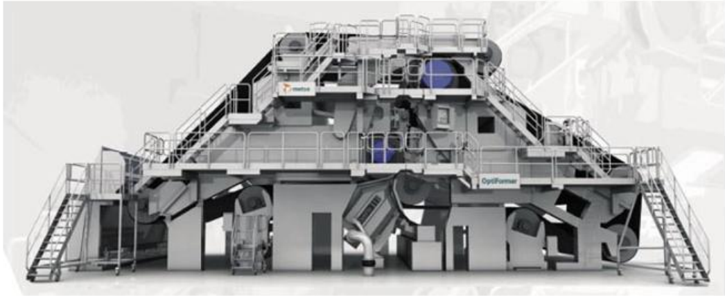
Figure 3.2.1.3 Gap former—one of three kind of web forming section. (Knowpap, web forming)
