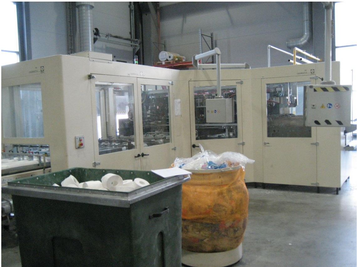
PICTURE 2. Körber Paperlink A5T in converting line 1
