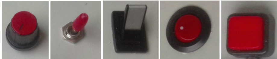
Figure 23. From left to right: potentiometer, toggle switch, on/off switch, rocker switch and push button (Juan Pedro Gimenez 2014).
