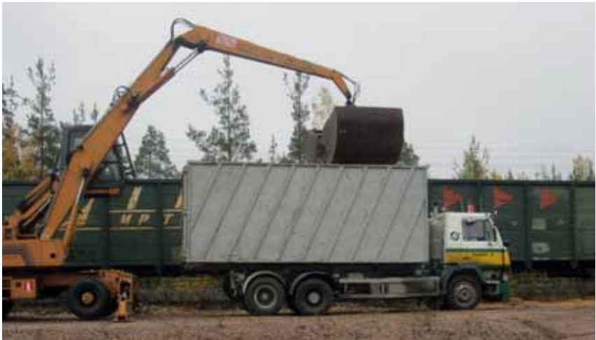
PICTURE 5. Transfer from a railway wagon to a truck in the Kurkvuori terminal, Finland (Lahtinen).
