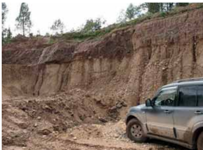
PICTURE 4. Stony material for road pavement under a two-meter layer of clay (glina) in Tikhvin (Greis).
