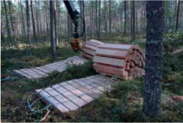
PICTURE 3. The first tested duckboard mat (Kontinen 2010).
