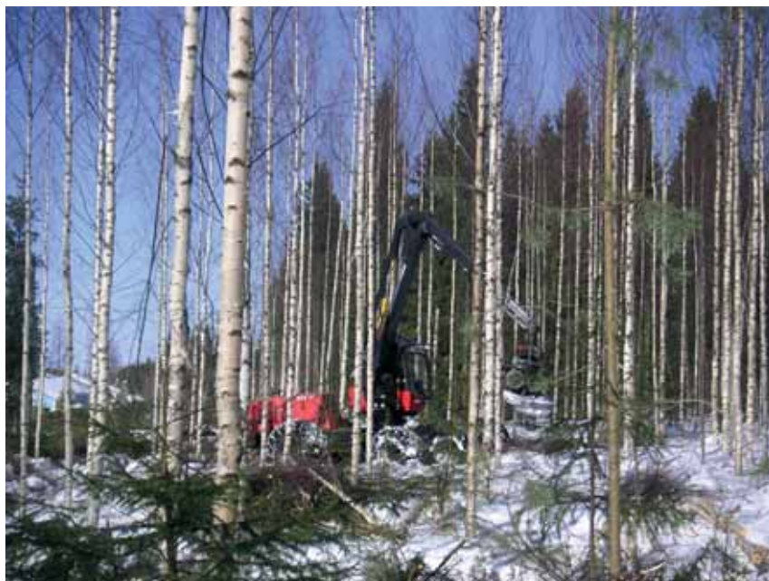
PICTURE 3. First thinning of a birch stand done by a medium sized single-grip harvester (Leinonen 2010).
