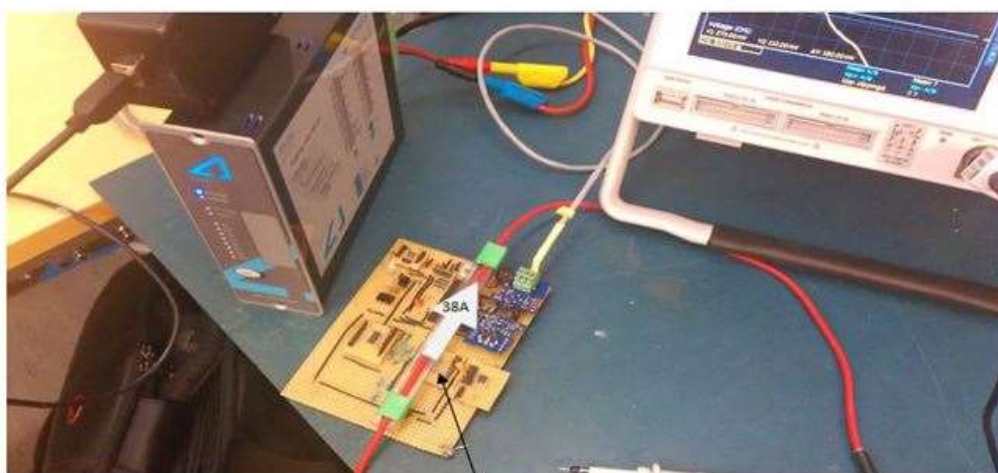
2 Axis AMR low magnetic field sensor (about 4 mm below conductor)
