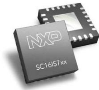
Figure 13: A I2C or SPI to UART or IrDA or GPIO bridge circuit [19]
