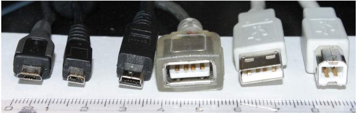
Figure 7: Types of USB connectors left to right (ruler in centimeters): micro-B plug, UC-E6 proprietary (non-USB) plug, mini-B plug, standard-A receptacle (upside down), standard-A plug, standard-B plug
