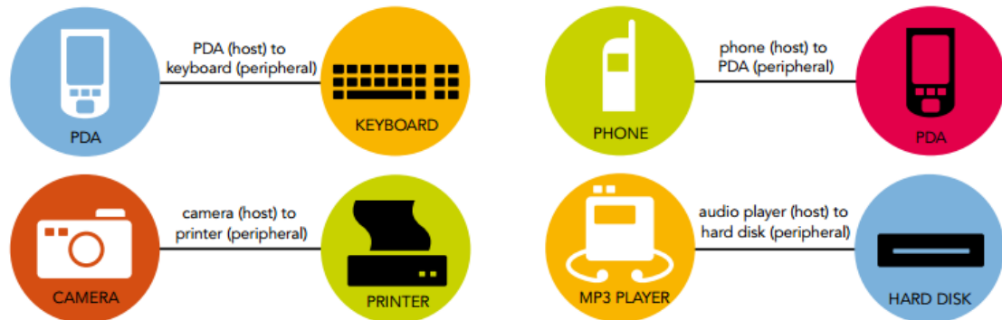
Figure 8: OTG enables point-to-point connectivity between peripherals without a traditional PC host. [11]
