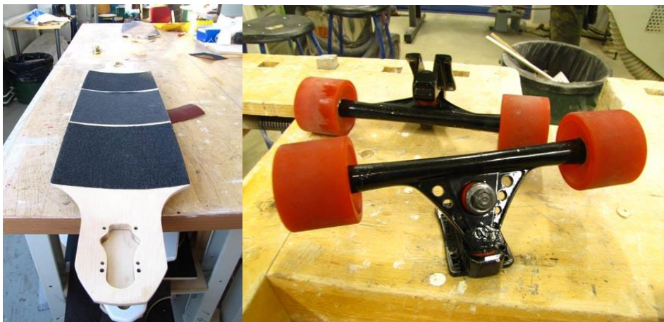
Picture 9. A deck with a grip and longboard trucks with wheels.
