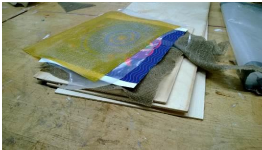
Picture 2. All the layers of a Lavia longboard.
