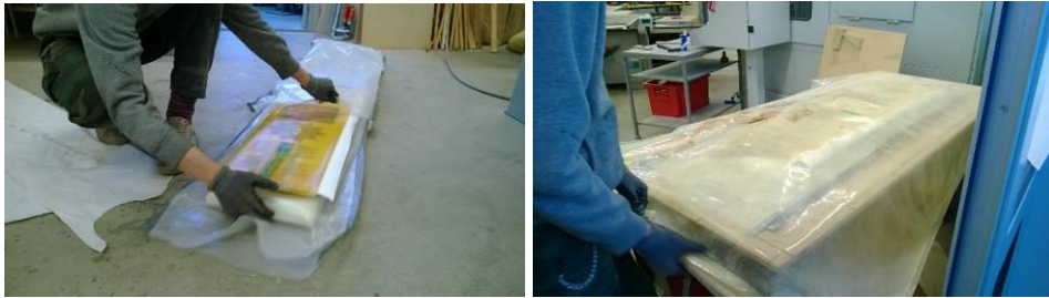
Picture 5 and 6. Putting the board into the bag and vacuum machine for overnight.
