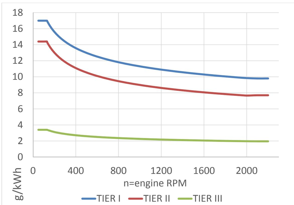
Figure 1 NO<sub>x</sub> emission limits for different Tiers as a function of the engine speed (By author)
