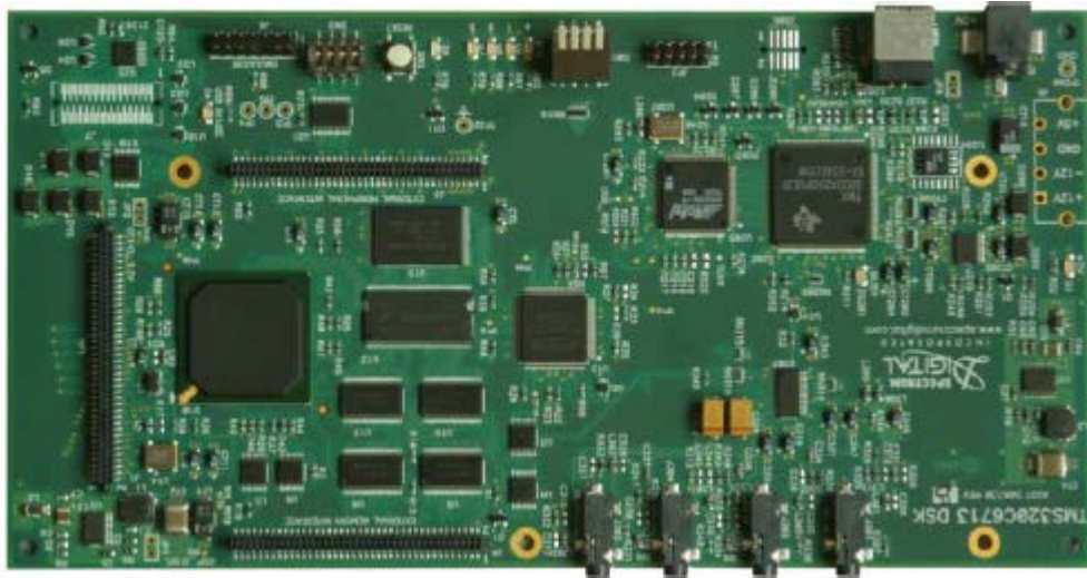
Kuvio 35. Texas Instruments TMS320C6713 Development Start Kit
