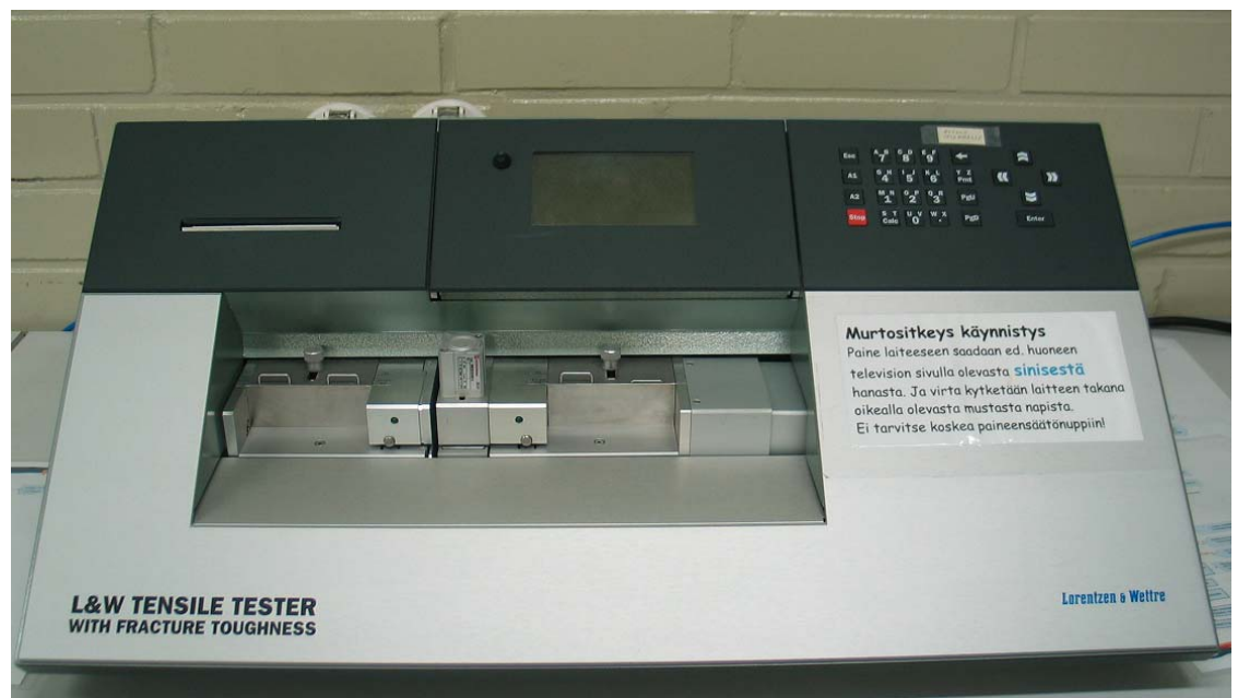
Figure 21 L&W tensile strength and fracture toughness meter
