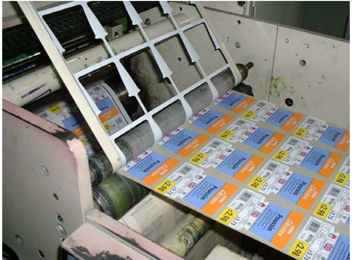
Figure 15 The waste matrix is removed against a cylinder /12/
