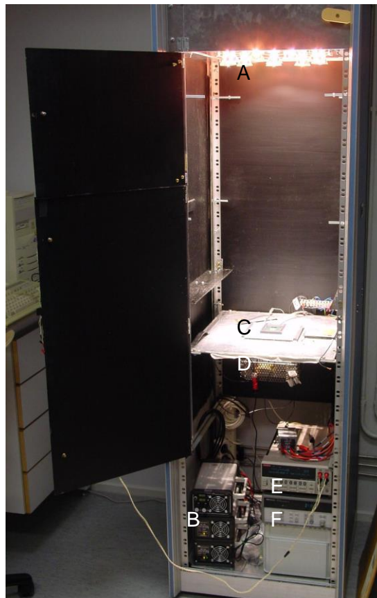
Figure 26. The solar simulator at the New Energy Technologies Group at Aalto University.
