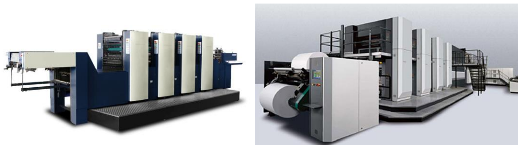
Figure 23. Sheet-fed printing. Reprinted from Qingdao 2FC Trading (2015) [85] and Web printing. Reprinted from Baldwin Technology group (2004-2014) [90].
