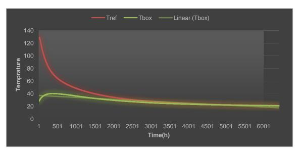
Figure 9: Time versus temperature plot for TEP's box-type solar cooker
