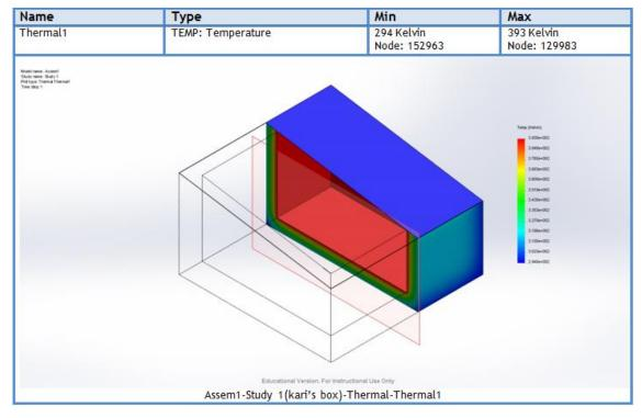
The improvement in insulation of TEp ry's box-type cooker can further be seen on the thermal simulation images shown in Figure 11 and Figure 12,
