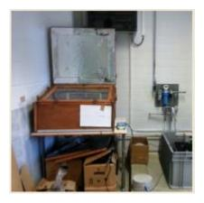
Figure 2. TEP ry's box-type solar cooker
