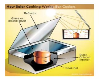
Figure 1. Box-type solar cooker (HowStuffWorks, 2009)
