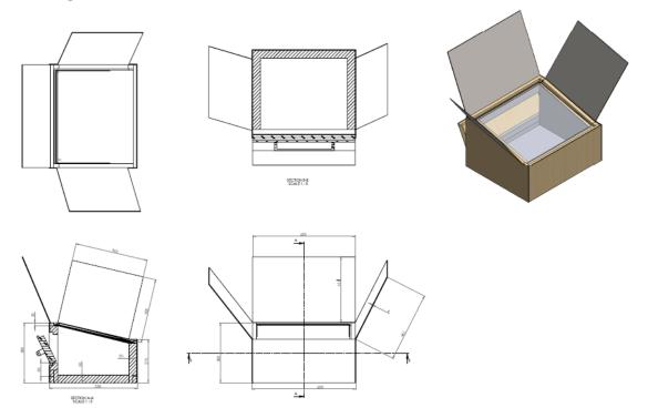
Appendix 1. TEP ry's box-type solar cooker SolidWorks CAD generated assembly design
