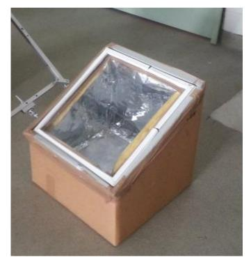
Figure 4. Experimental rig of the Metropolia 1 box-type solar cooker
