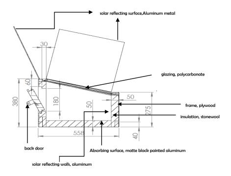
Figure 3. Sectional schematics of TEP ry's box-type solar cooker
