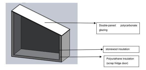
Figure 5. Sectional schematics of Metropolia 1 box-type solar cooker
