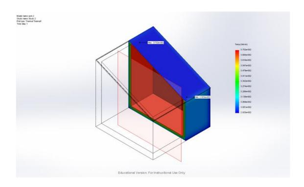
Figure 12. Thermal simulation results for Metropolia 1 box-type solar cooker
