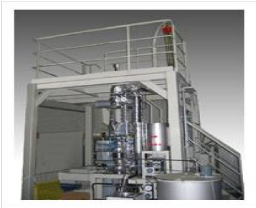
Figure 4: Supercritical reactor for plastic waste (Nikkiso co, ltd, 2000)
