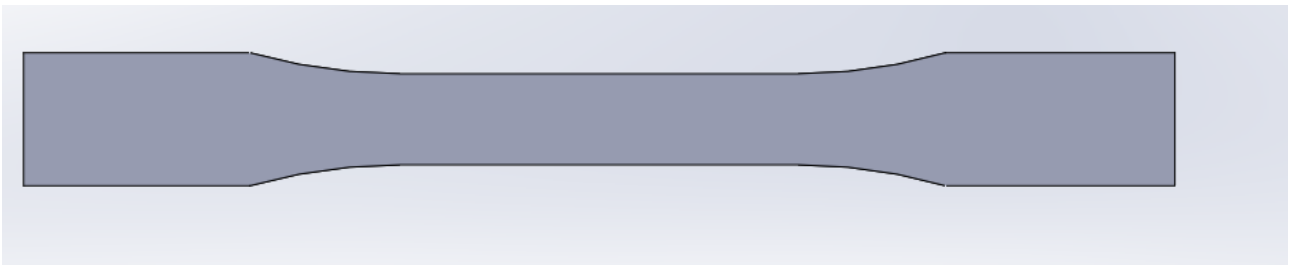
Figure 14: Dog-bone diagram drawn with solid works software
