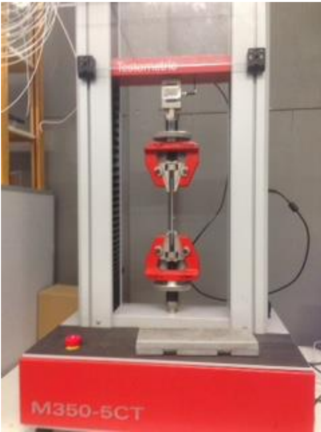
Figure 15: Dog-bone mounted on a grip being tested with a testometric tensile testing machine (Arcada plastic technology laboratory, January 2015)
