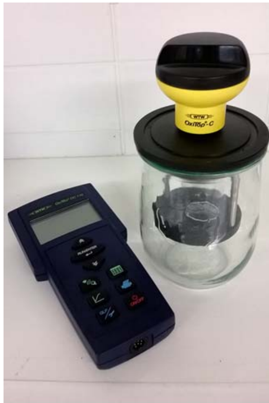
PICTURE 1. OxiTop® measuring vessel, lid, measuring sensor and controller
