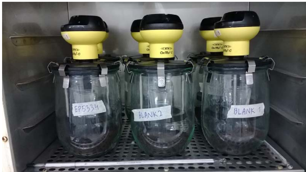
PICTURE 8. Soil respiration samples in incubation cabinet
