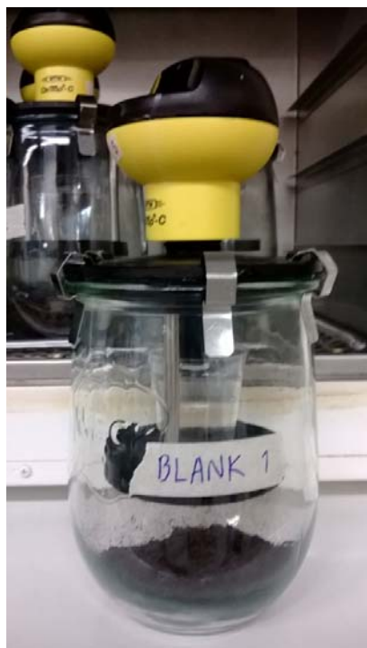
PICTURE 7. Blank sample in OxiTop® measuring vessel
