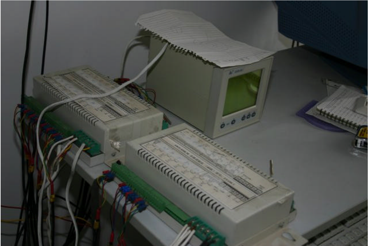
Picture 4-2, 64-chanel temperature measurement unit + screen
