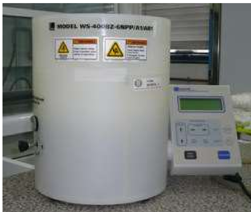
PICTURE 2. Spin-coater machine used in the experiments
