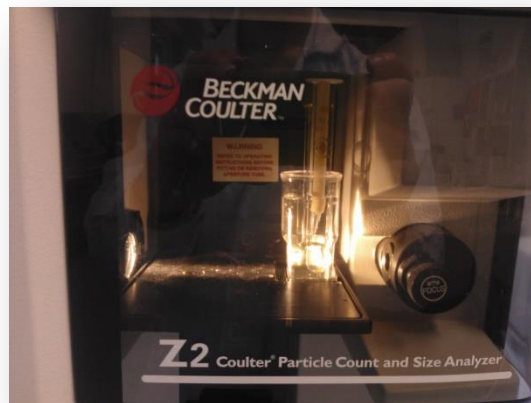
Figure 14: Beckman cell counter (Beckman Coulter, Type: Z2) in operation - used in this studies’ laboratory tests
