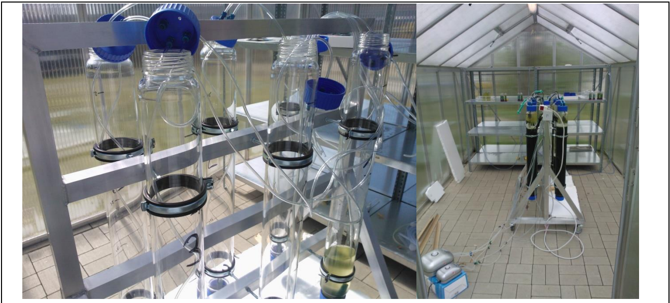
Figure 9: Tube reactors used during the Greenhouse phases. On the right picture the greenhouse, reactors (middle) and aquaristic pumps (left bottom).
