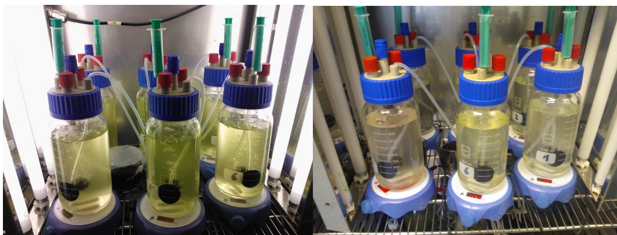
Figure 28: Starting (on left) and 2 days old cultures (on right). 18 ml heavy metal solution (300 \mu g/L Pb, 30 \mu g/L As, 30 \mu g/L Cd and 30 \mu g/L Hg) was added to each cultures (n=6, pH3, t= 3 days). The color change of death cultures is visible on the right picture.
