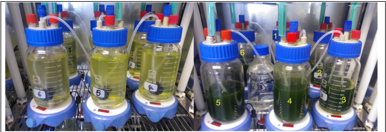
Figure 34: Fresh 0 day old cultures (on left) and same cultures after 14 days (on right). 18 ml heavy metal solution (300µg/L Pb, 30µg/L As, 30µg/L Cd and 30µg/L Hg) was added to each cultures (n=6, pH5, t= 14 days).
