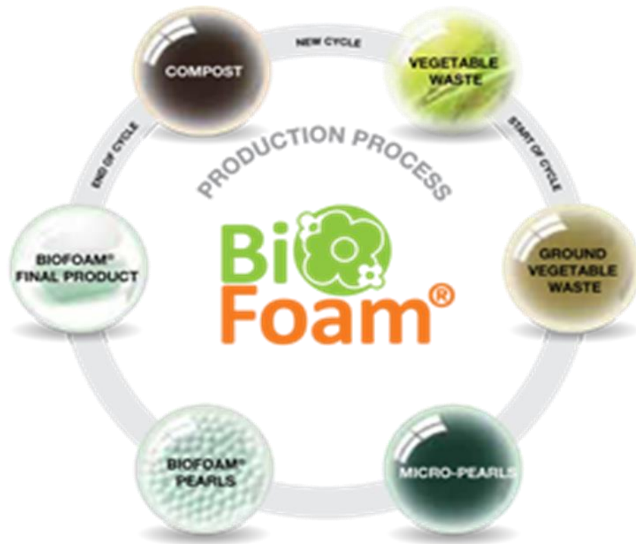
Figure 7.1 Production process of BioFoam (Biofoam, 2014)
