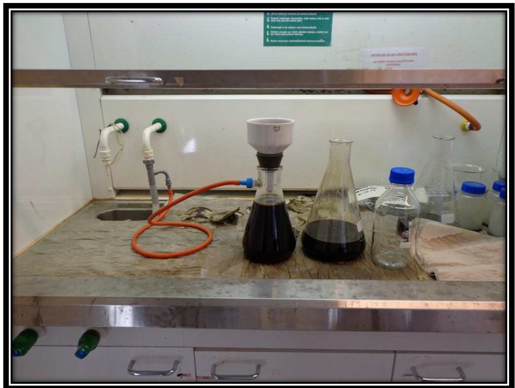
Fig.11 Wastewater from Kujala during filtration.
