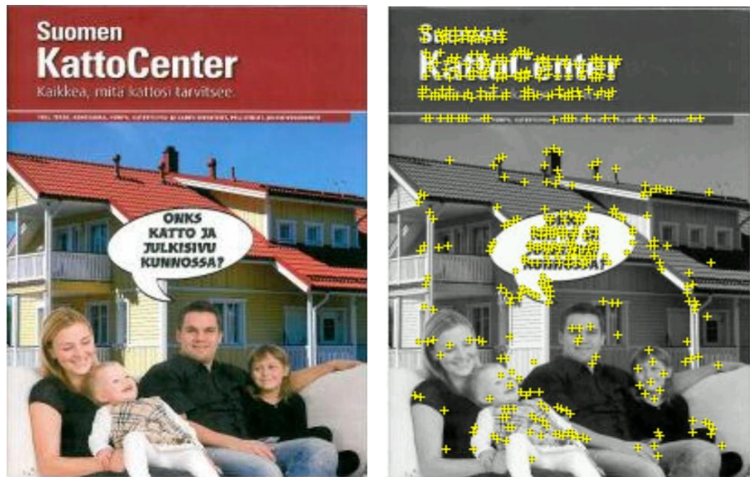
Figure 15: -a) KattoCenter image target -b) KattoCenter image target with features used for tracking
