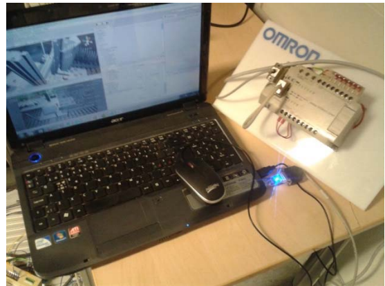
Figure 13. A laptop is connected to PLC
