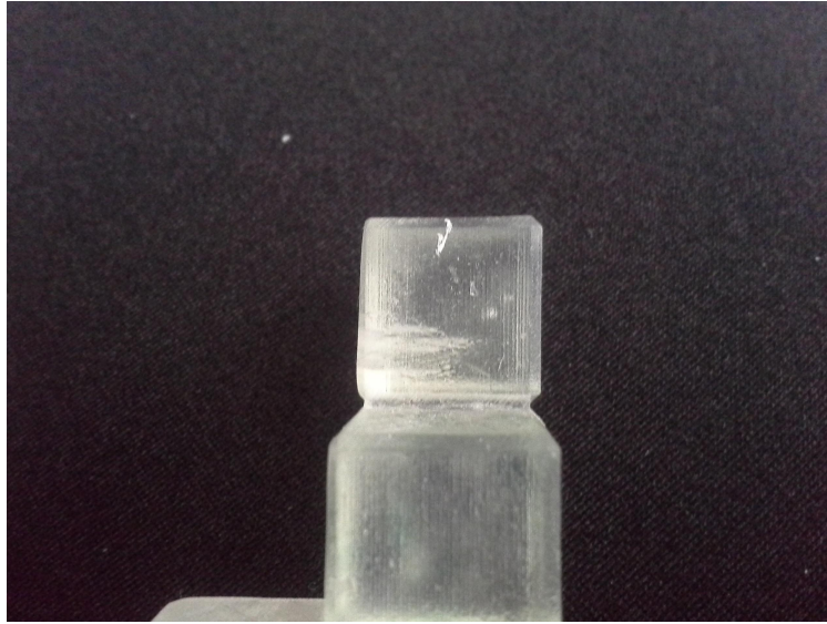
Figure 39 Picture of the skewness of the cubes printed with 0,1mm layer thickness. Part was oriented 45 degrees, suggesting either improperly tuned z-axis or some other fault.
