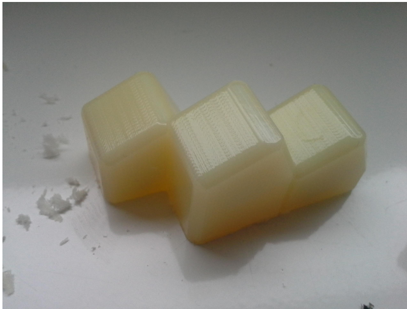
Figure 42 The same cuboid before support removal, covered in support material. The support material is fragile and sticky wax like substance. It is difficult to remove with a knife and best done on the WaterJet machine supplied by Stratasys.
