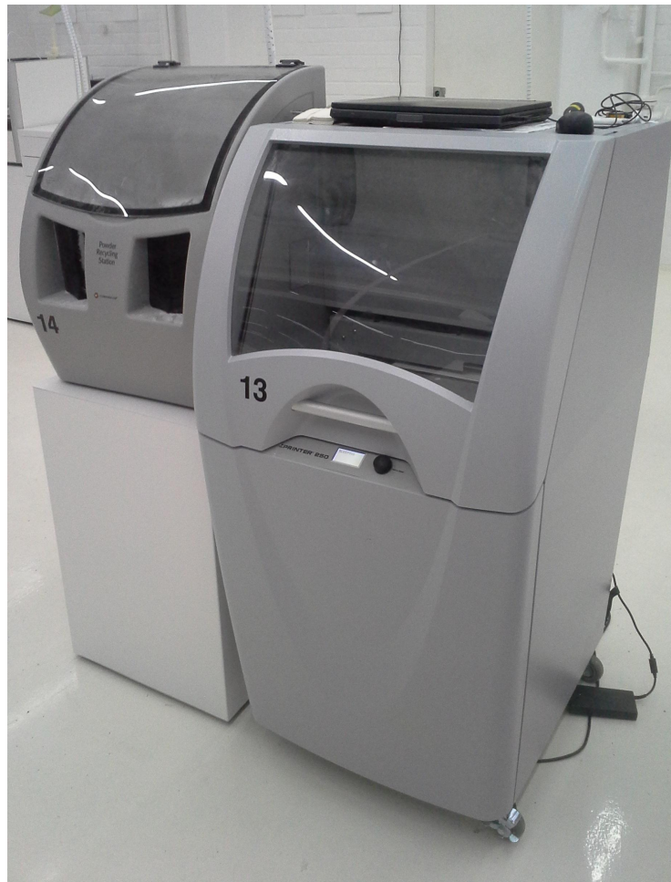
Figure 23 The Zprinter Powder printer pictured. Notice the powder recycling station next to it.
