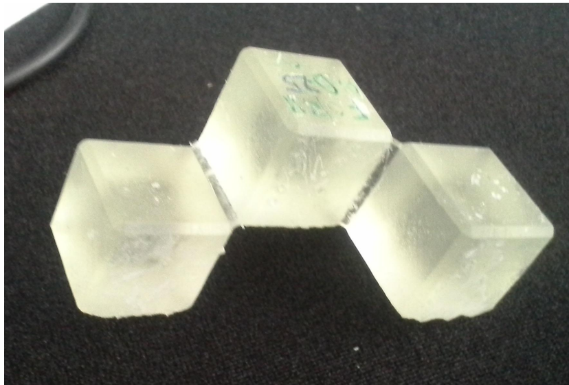
Figure 40 Cuboid printed with Form 1 with 0,025mm layers. Notice the imperfections inside the cubes and the bottoms where the support structure was built.
