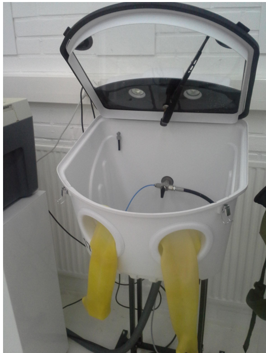
Figure 21 The WaterJet washing station. Not pictured: pressure water pump (standard hardware-store type) and foot pedal for controlling the pressure.
