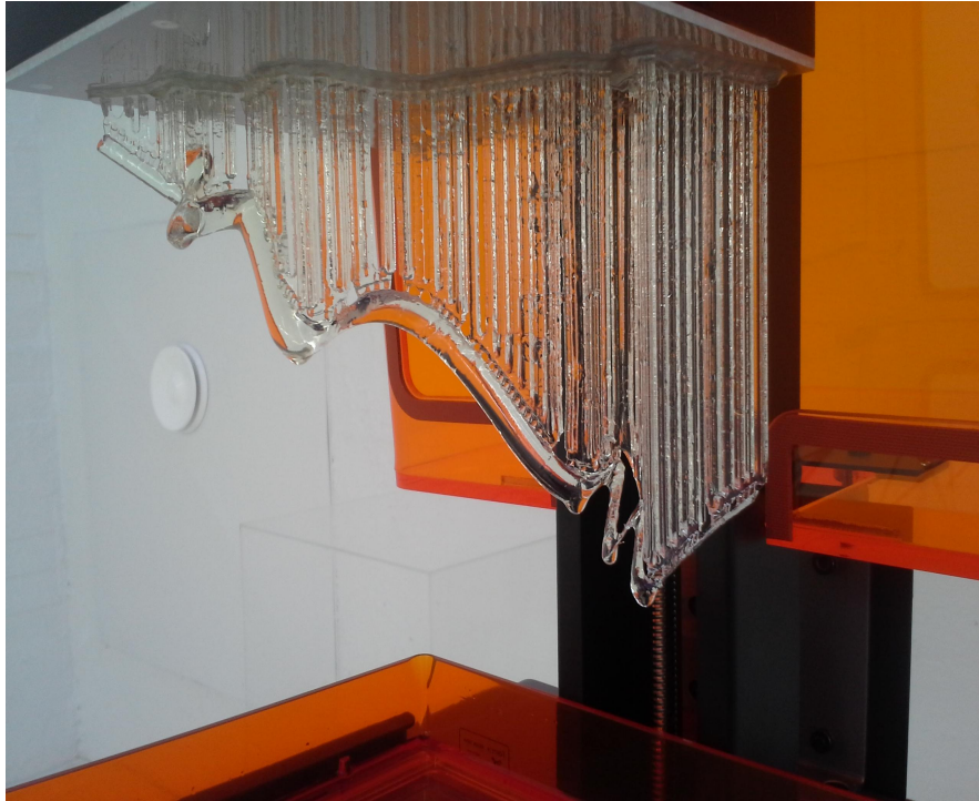
Figure 16 An art piece printed with the Form 1. The printer works best with small surface area pieces, and doesn't have problems producing fine details if they are properly supported. The pictured piece was broken during support removal, requiring gluing. Also sanding was needed for surface finish
