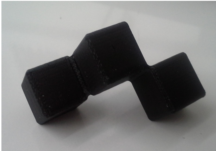
Figure 35 Cuboid printed with uPrint SE Plus.
