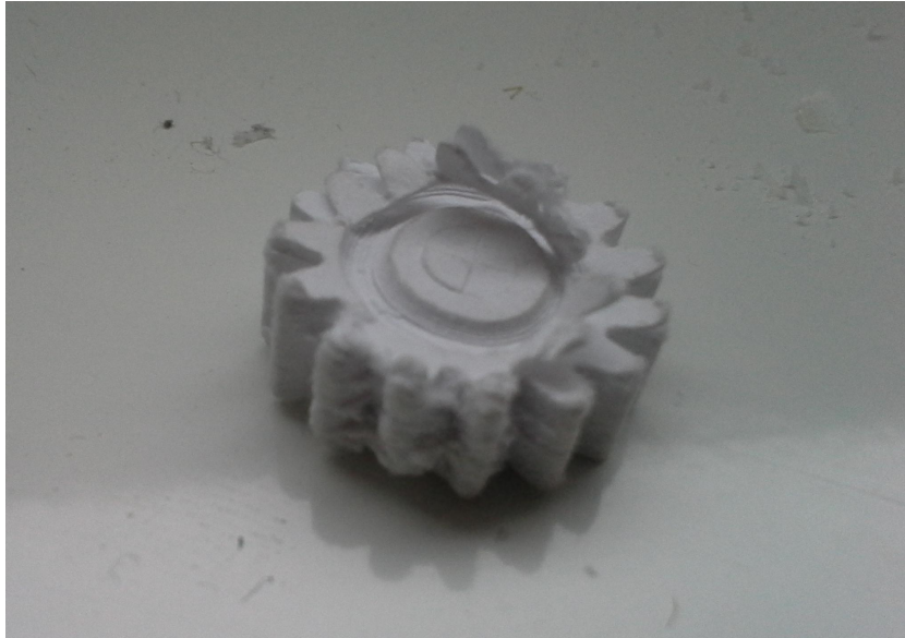
Figure 27 A small gear of approximately 10mm in diameter, printed with the Mcor, showing easily separable layers.
