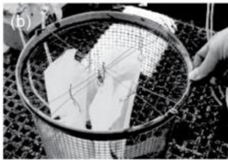
PICTURE 3. Passive samplers designed for water column deployments: polyethylene and polyoxymethylene strips fastened to the interior of a fish trap [8]
