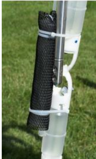
PICTURE 7. Deployment of the Snap Sampler [15]
