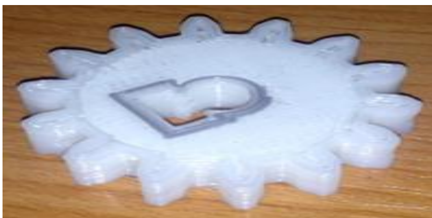
Figure 19 : Test piece (Gear ring) provided by minifactory with the 3D Printer
