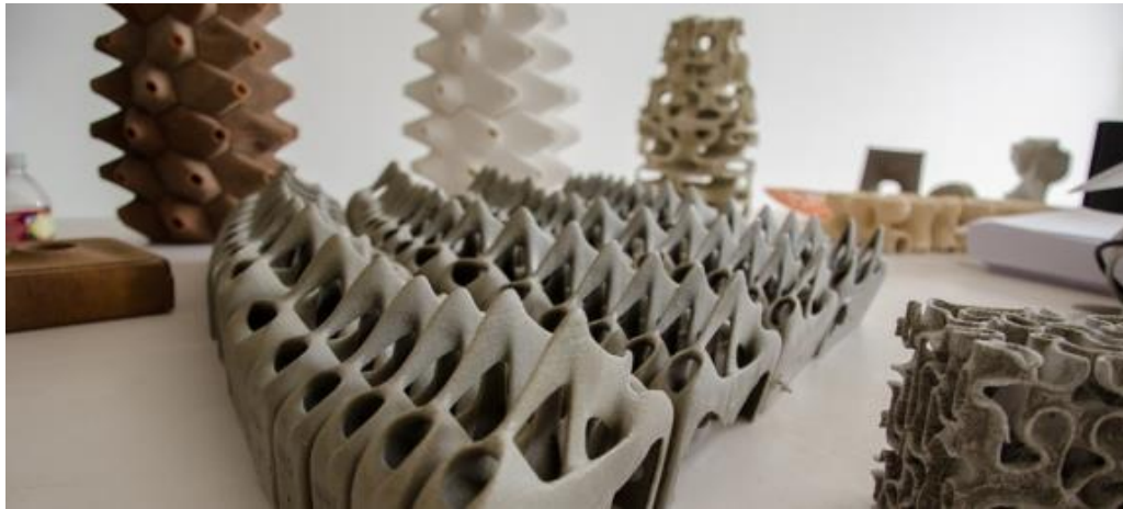
Figure 13: 3D printing using concrete (can withstand 4000 pounds pressure) (27)
