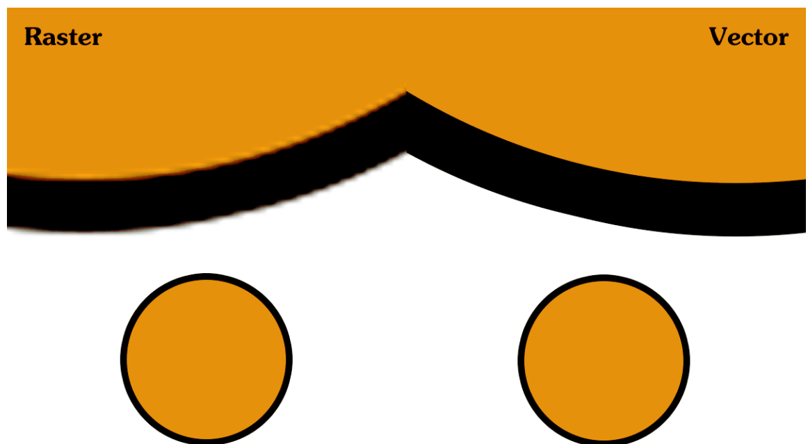
Figure 5. Comparison of identical balls both in raster and vector graphics, which are then scaled six times bigger.
