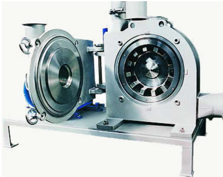
Figure 6: Hosokawa Alpines impact mill ( http://www.hosokawa.co.uk/alpine.php , figure text Aleksii Puurunen)
