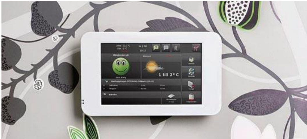
Figure35: Smart interface of heating system.
