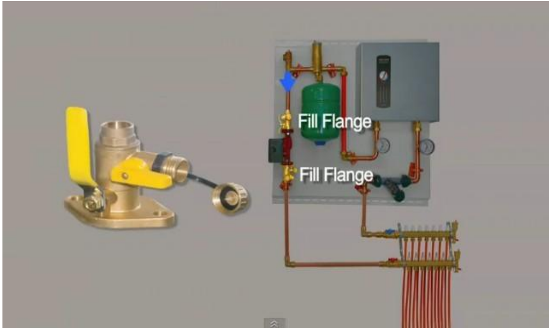
Figure6: Fill Flange in a heating system.
