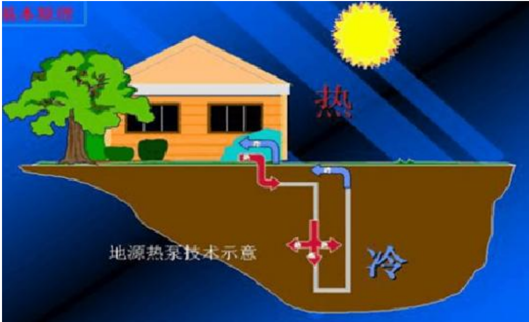
Figure18: Ground source heat pump technology schematic diagram in the winter.
