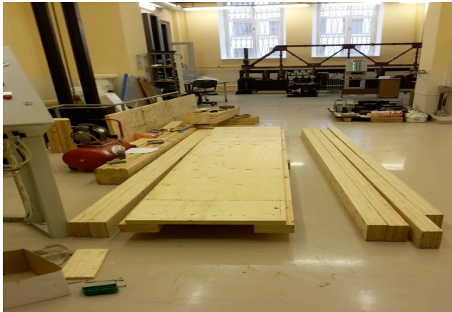
Figure 19. LVL web and flanges.
