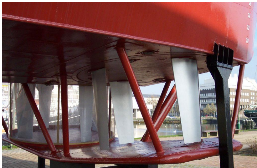
Picture 4 Voith Schneider propeller (The Art Of Dredging 2015)
