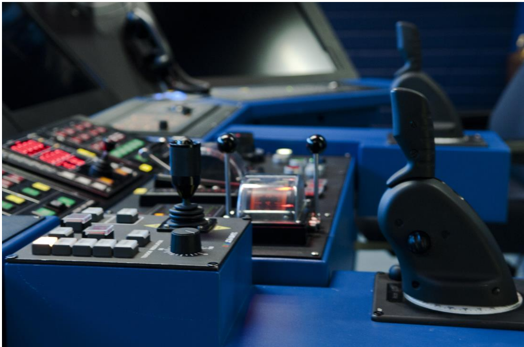
Picture 8 The operation devices of tug simulator of Aboa Mare, the control device of tension winch can be seen at the left. (2015)
