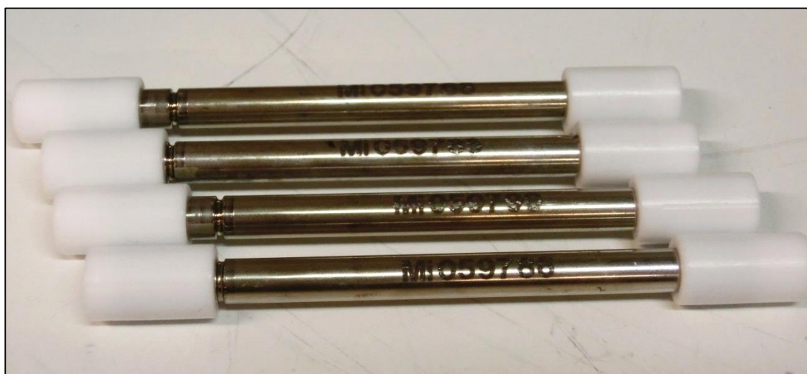
Figure 8. Tenax TA tubes manufactured from Marke International. Each tubes are labeled with numerical code. The side with a ring of groove is the head of the tenax tube.
