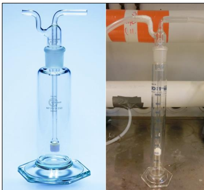
Figure 11. Measuring cylinder coupled with Dreschel bottle head (sinter porosity grade 0) (Dreschel bottle heads, camlab, n.d.).
