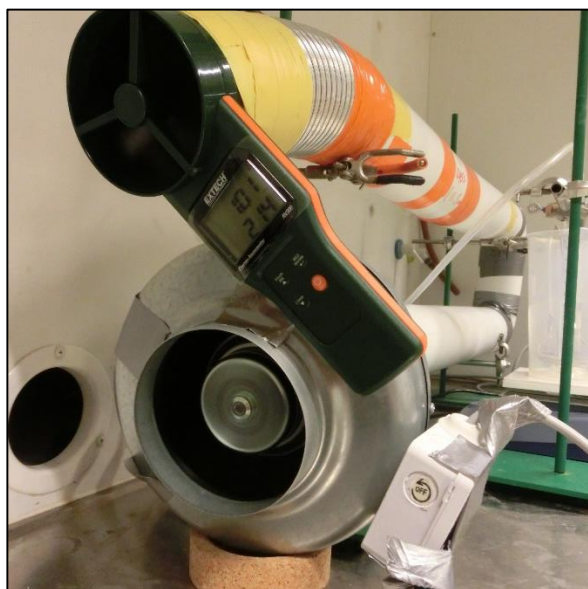
Air speed meter used to control the fan.
