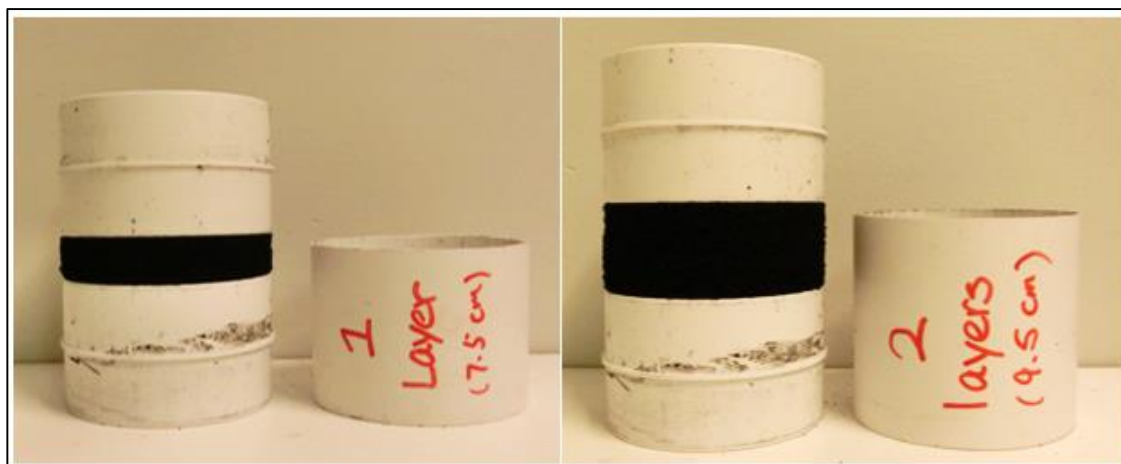
Figure 12. IAC filters with one layer and two layers. IAC (black part) is placed in between two PVC pipe joints when fit into the corresponding PVC cylinders. One-layer and two-layer IAC filter have length of 7.5 cm and 9.5 cm. Three-layer IAC filter has a length of 11.5 cm.
