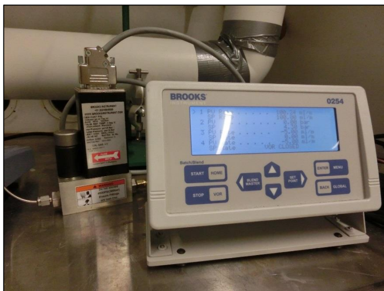
Air flow meter used to control the nitrogen gas flow. (Model: Brooks Instrument Delta Smart II Mass Flow (left) and Brooks Instrument 0254 (right).)
