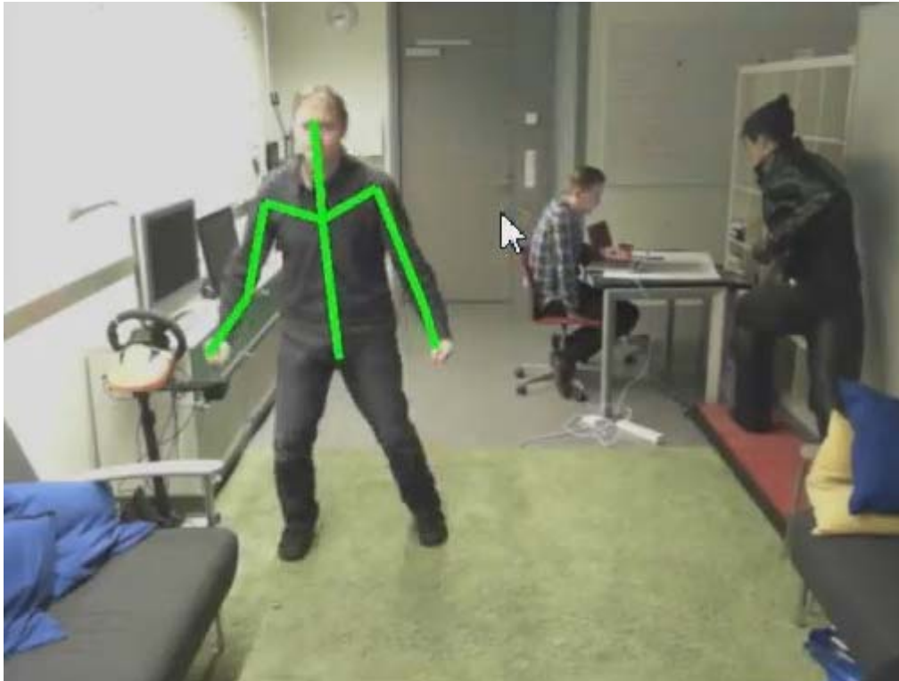
Picture 4. Skeleton generated by Extreme Motion overlaid on the input color image.
