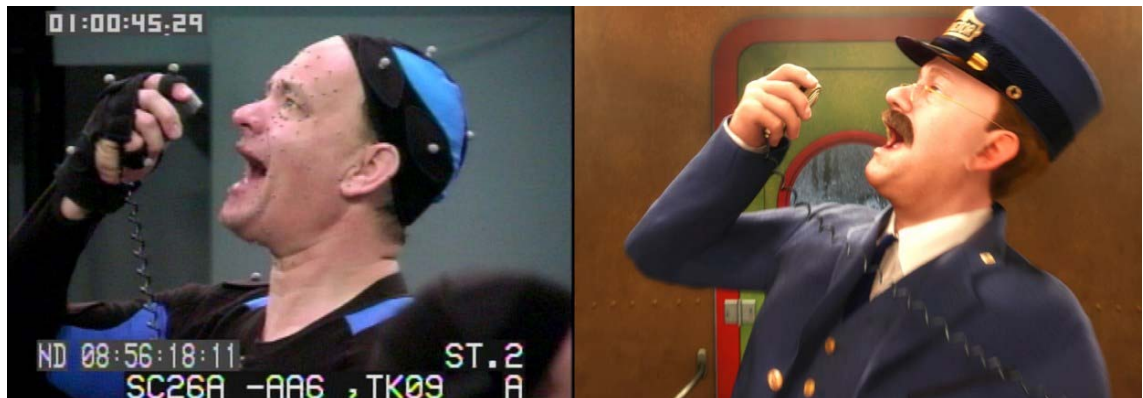
Picture 1. A motion capture setup using IR markers, side-by side with the resulting computer generated "shot". (Bredow etc, 2005, 3)
