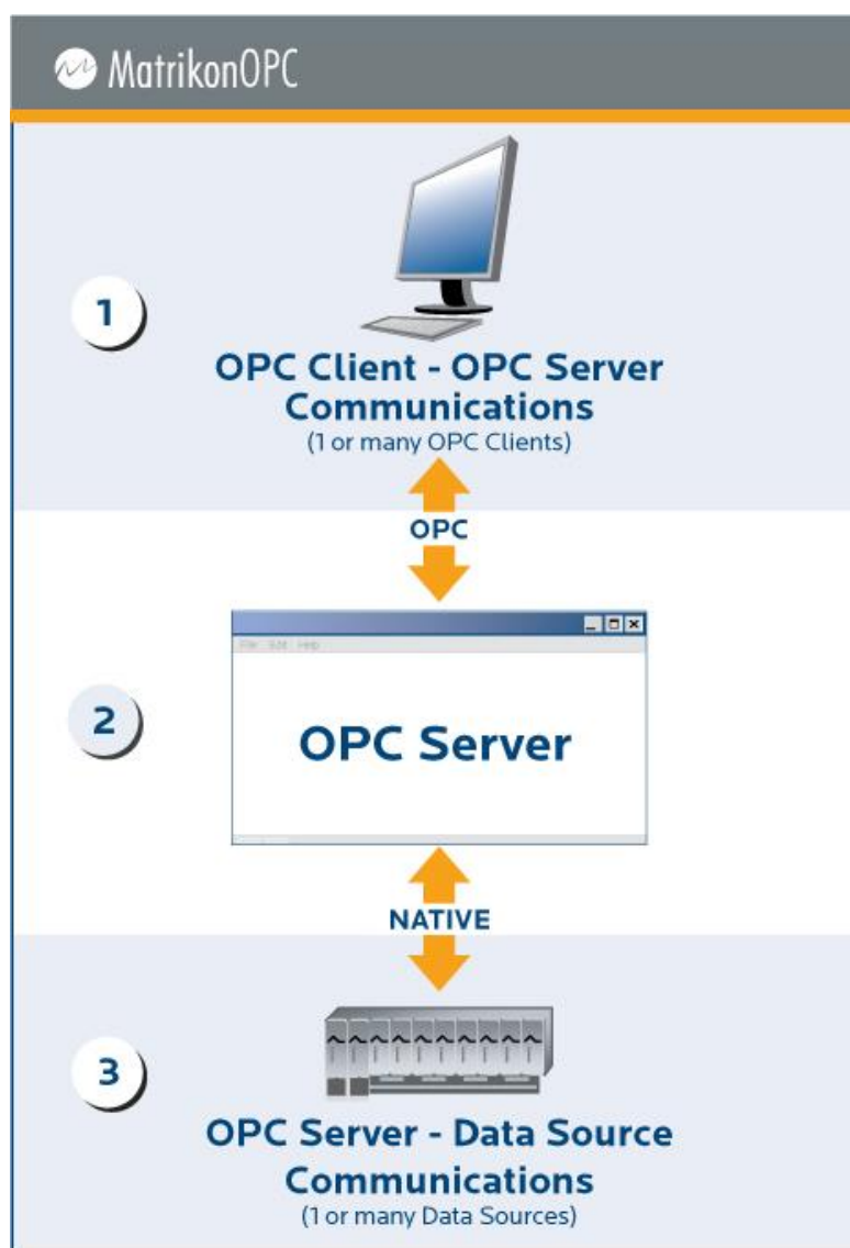
Figure 6. The connection between OPC client, server and hardware.
