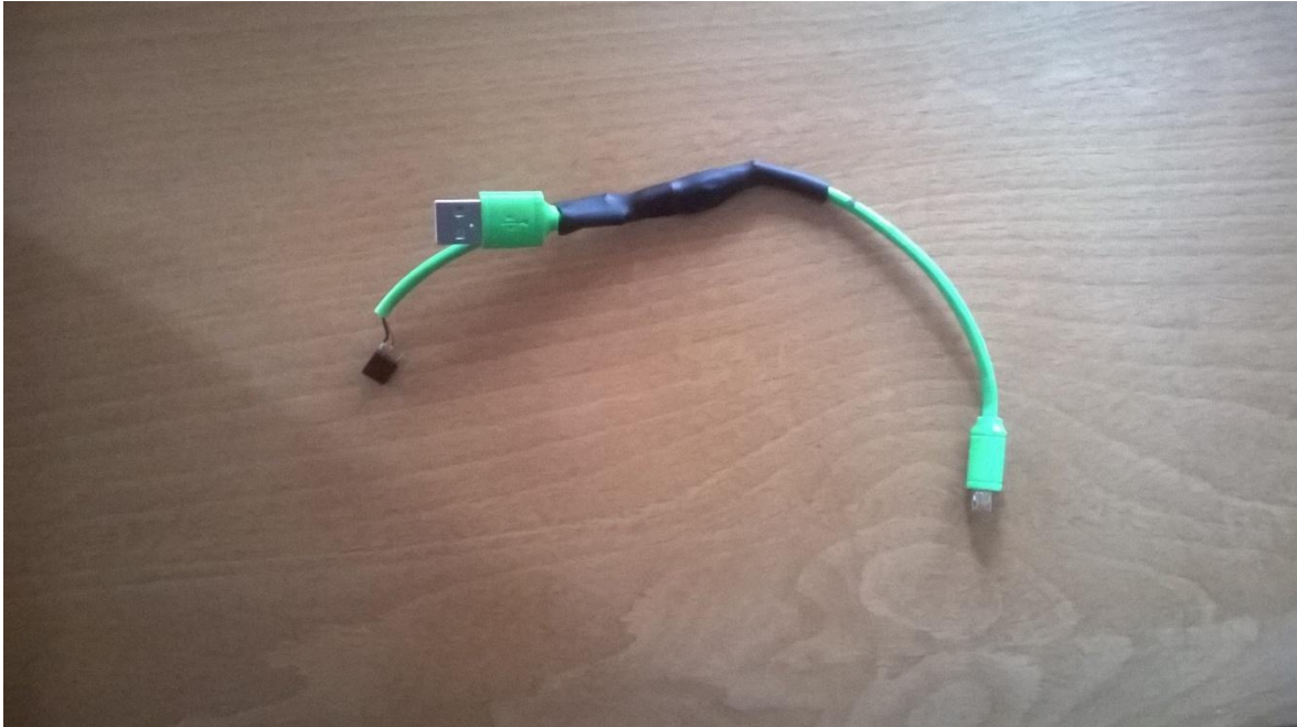
Picture 3: The finished Raspberry Pi power cable. Heat shrink has been added to protect the soldering.
