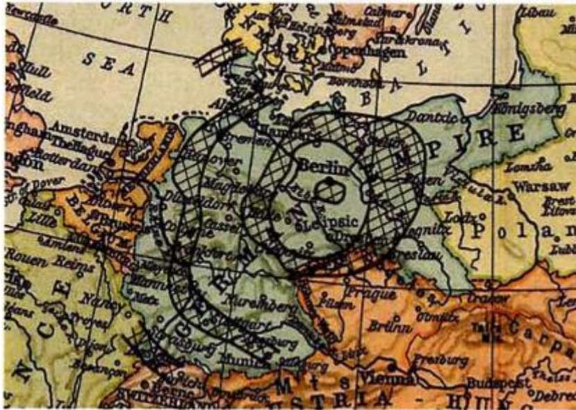
Figure 21: An explosion in Kummersdorf (South of Berlin) on 18 th December 1925 had sound propagating unusually far, the crossed regions signifying where the explosion was heard. The pattern is a clear result of sound waves hitting a temperature inversion and then being refracted back to the ground, which it in some cases reflected off of, sometimes even several times. [37]
