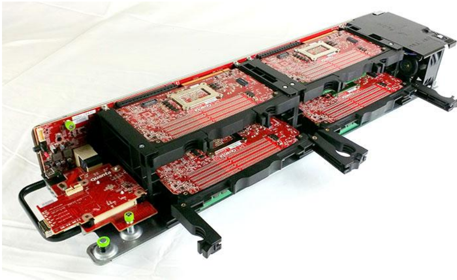
Figure 4: Facebook's "Yosemite", the world-first open source modular chassis servers. Reprinted from Hu Li, Facebook (2015)
