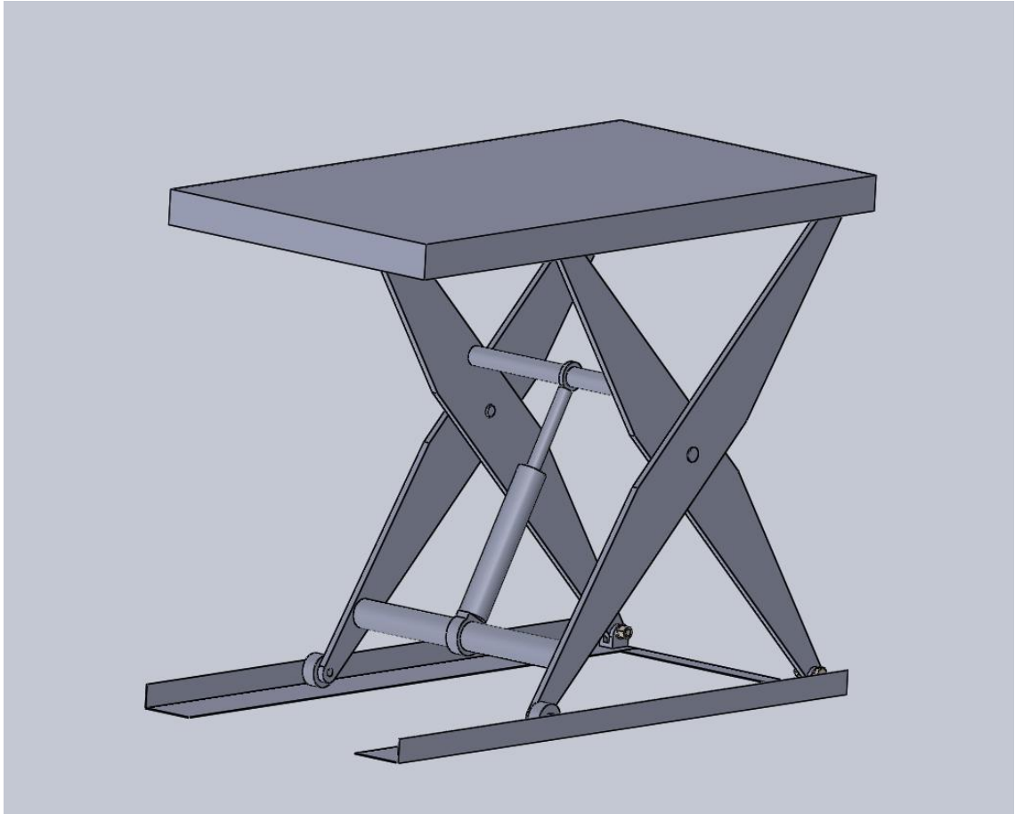
Figure 9.5 3D view of the lift
