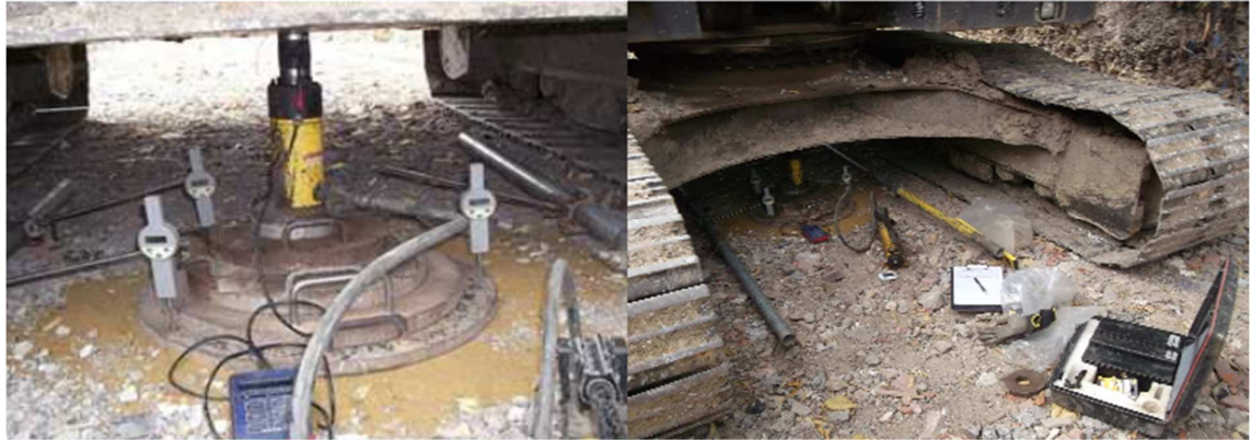
Figure 43: Plate bearing test setup. ( Plate bearing test )
