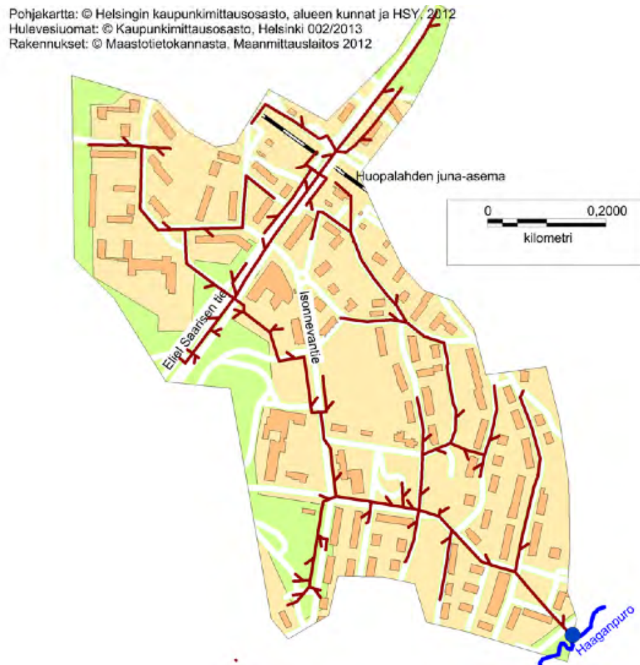
FIGURE 10. Map of the drainage area of the rainwater system (Airola et al. 2014)
