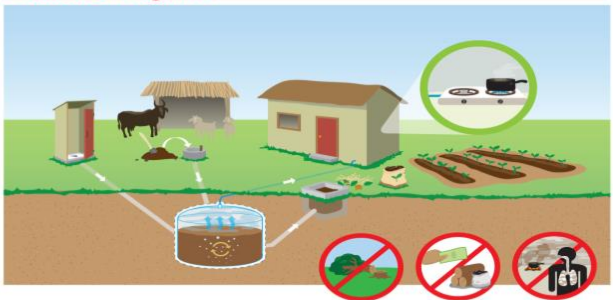
Figure 7- Typical Bio-Gas Generation System [20]
