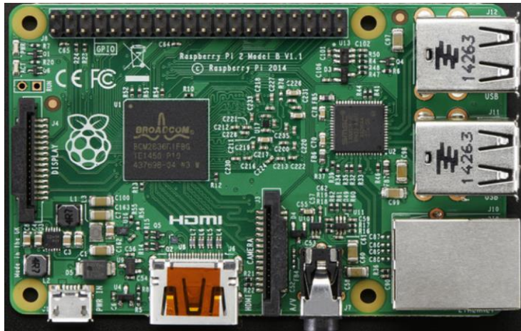
Figure 6. Raspberry Pi 2-model B. Reprinted from Adafruit [4].
