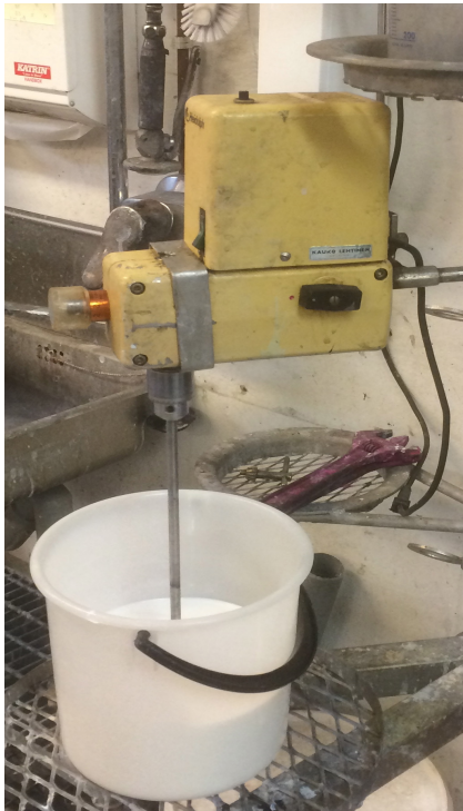
Figure 24. The Mixing of the binder solution.
