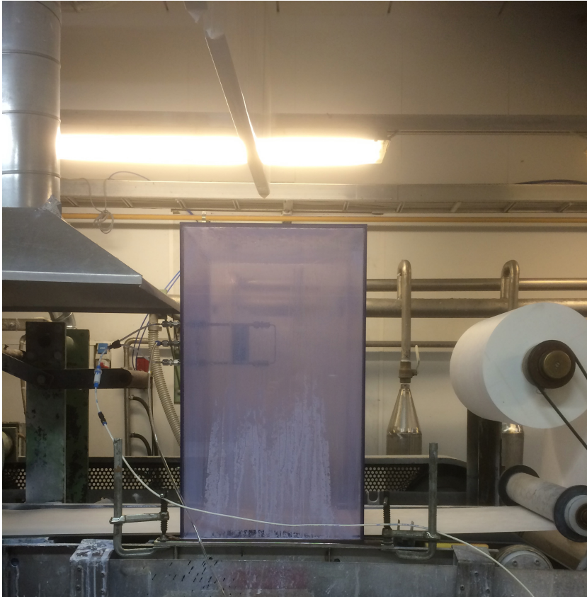
Figure 25. The aerosol coating unit on a forming wire.
