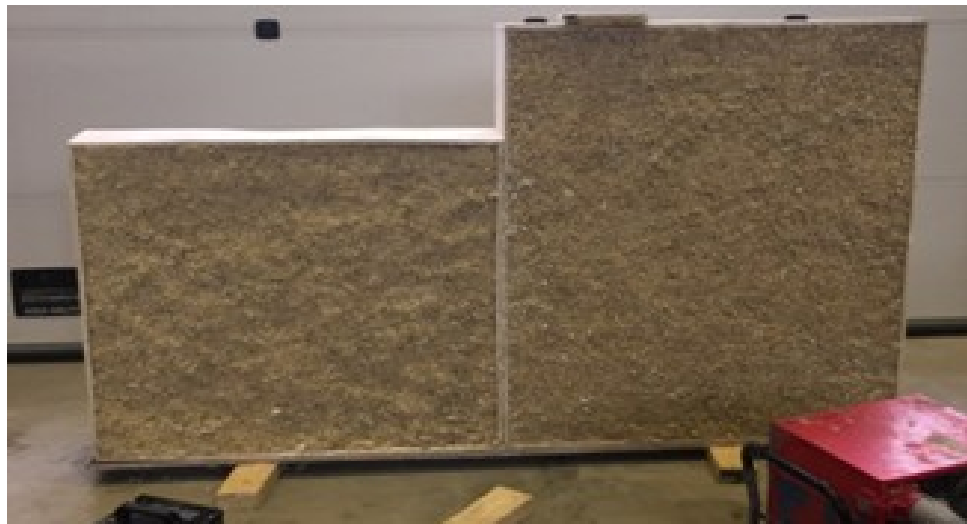
Figure 13 Wall - 2 after four days of casting in the HAMK SMC
