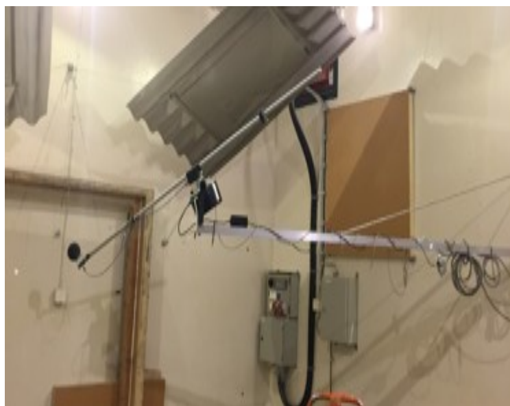
Figure 31 Highly sensitive Microphones to Measure Sound level in the laboratory
