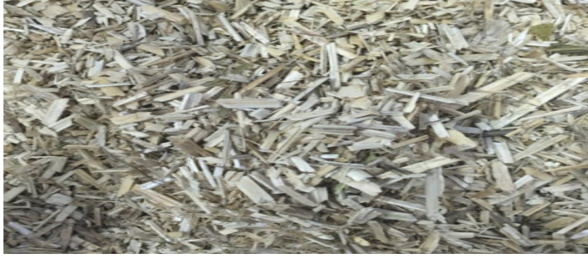
Figure 3 Hemp shives ready to be used as an aggregate (source: Hemprefine Oy)
