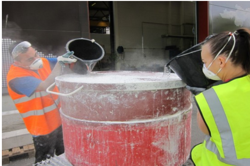
Figure 9 Mixer filled with shives, lime and water in the Laboratory
