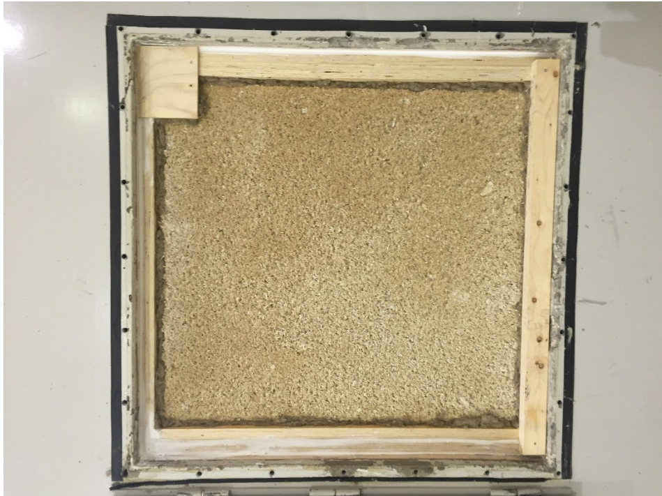
Figure 30 Set up of wall sample between reverberation chambers
