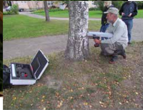
Investigation with a Resistograph- auger.
