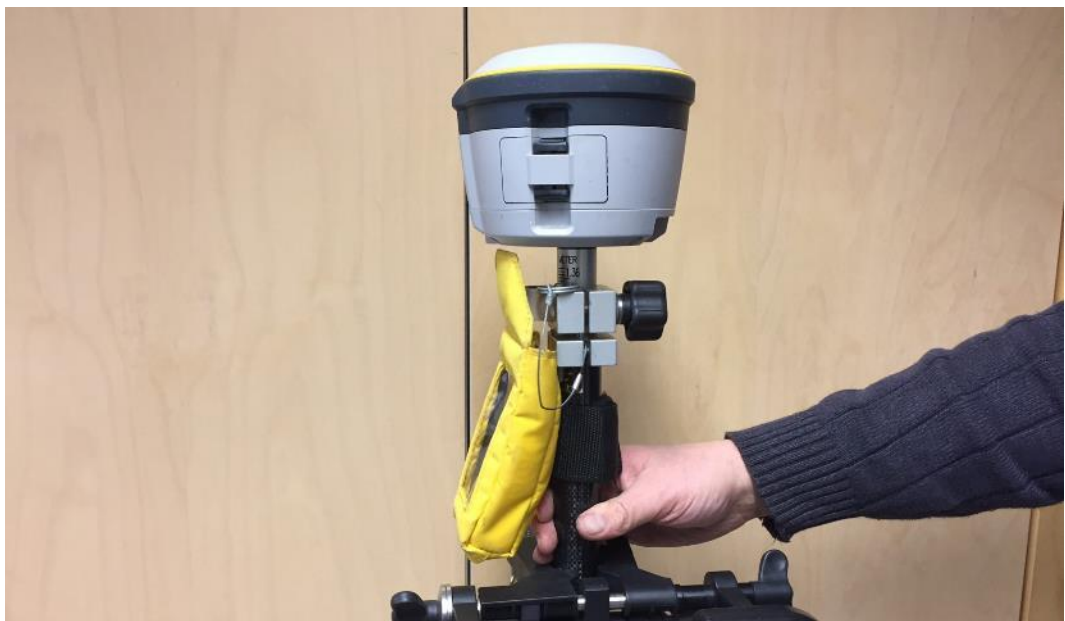
Figure 16. Trimble R2 GNSS –satellite receiver. The survey accuracy is in centimeters. (Katja Virtanen 2016)
