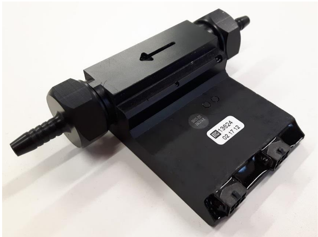
FIGURE 56. The final construction of the gas flow meter
