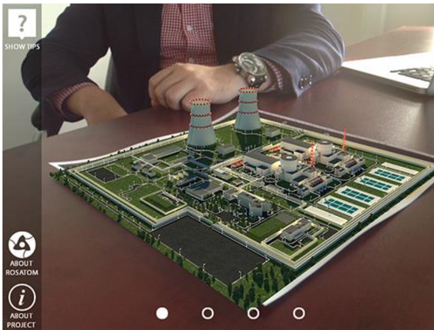
Figure 18. Miniature model of a power plant in AR developed on Vuforia's platform.
