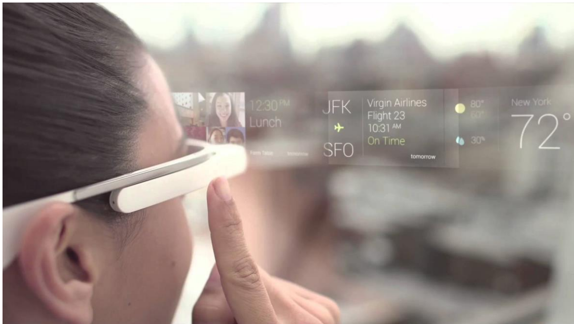
Figure 1. Google Glass Augmented Reality from 2013. Content is controlled by touch on the glass frame. A basic demonstration of projection technology. Field of view approximately 25 degrees.
