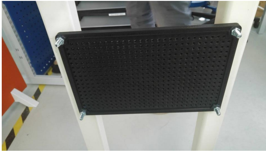
FIGURE 46. Bracket for electrical parts
