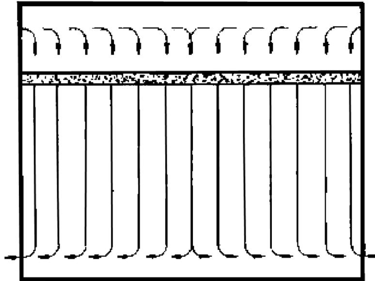
**Figure 6. Unidirectional downflow air distribution. /7/**
