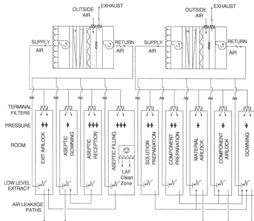
**Figure 1. Air supply and extract in cleanroom suite using the “closed door” solution /6/**
