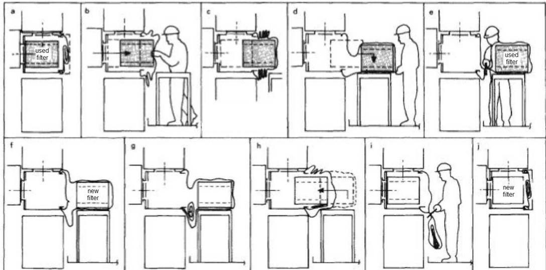
**Figure 8. Safe procedure of changing a filter. /7/**
