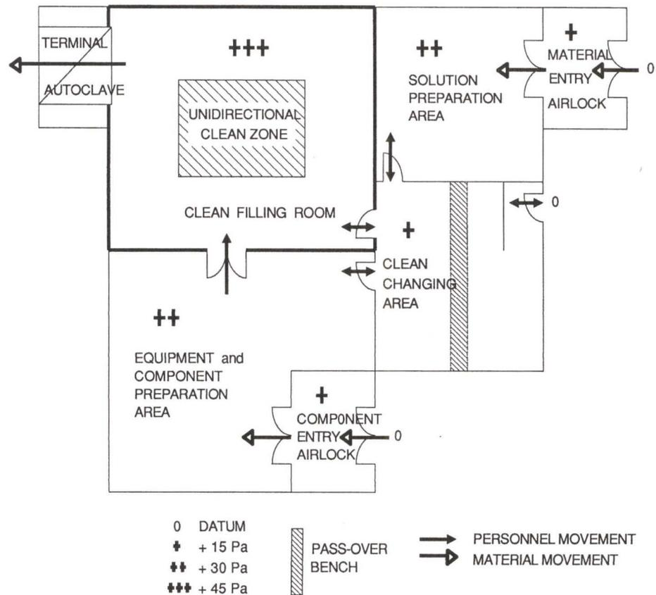
**Figure 3. Typical suite of rooms for terminally sterilized injectables. /6/**
