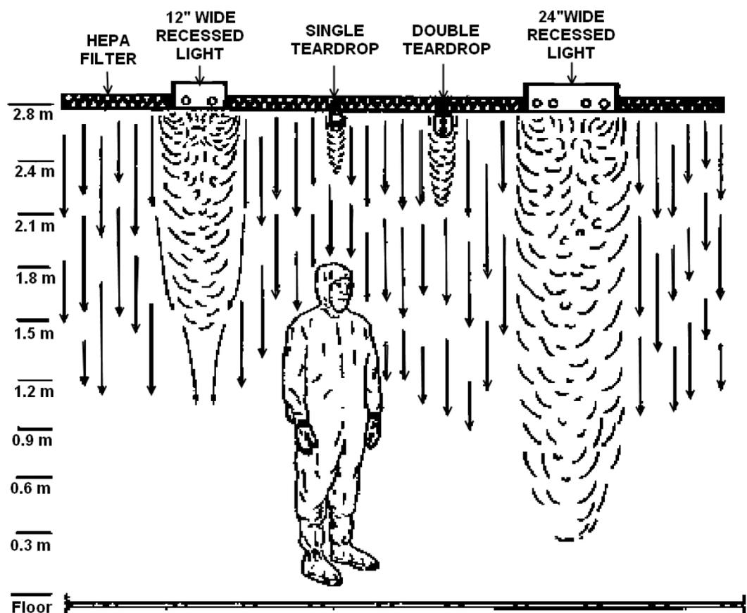
Figure 7. Obstruction cased turbulence in a laminar flow cleanroom. /7/
