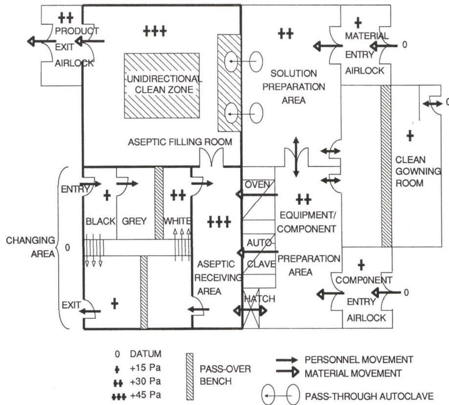
**Figure 4. Typical suite of rooms for aseptic filling. /6/**
