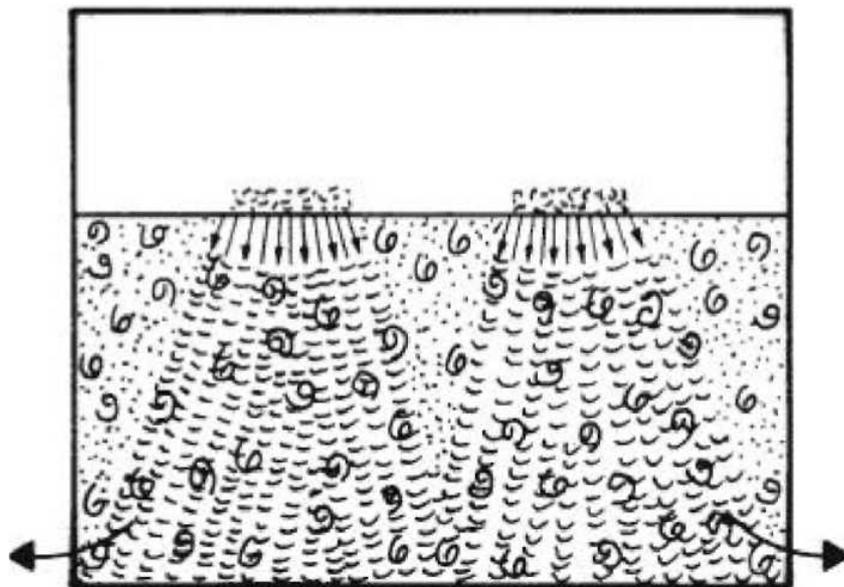
**Figure 5. Turbulent flow air distribution. /7/**
