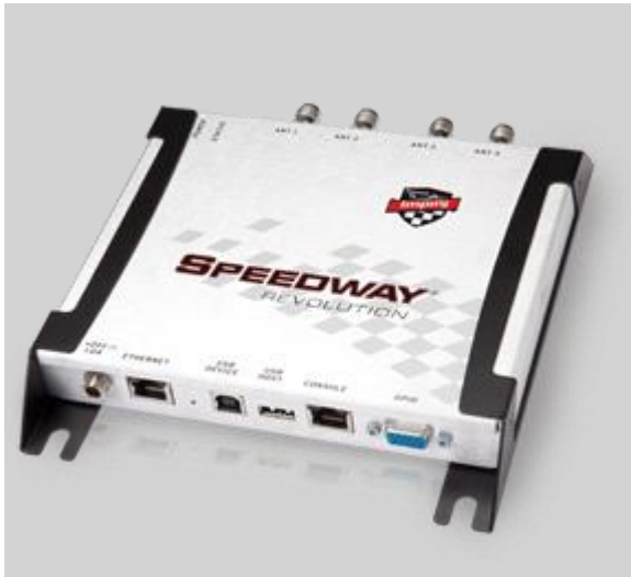
Figure 3: RFID Reader Device - Impinj Speedway Revolution R420 [6]
